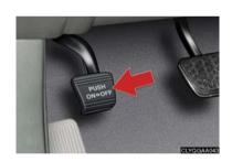
To set the parking brake: firmly depress the parking brake pedal.
