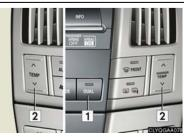
In DUAL mode, driver and passenger side temperature settings can be adjusted separately.
