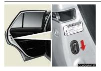
Setting the switch to the LOCK position prevents the rear doors from being opened from the inside.
