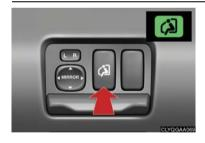
To turn the easy access mode on and off, press the easy access mode switch.
