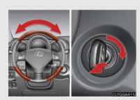
Turn the ignition switch while lightly moving the steering wheel from left to light.
