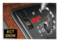
An indicator comes on when in snow mode. Press again to return to normal mode.
