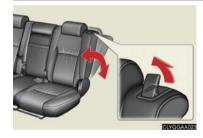
Pull the lever and tilt the seatback forward or backward.
