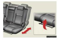
With the lever raised, slide the seat forward or backward.
