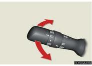
To engage the high beams, push the lever forward. To flash the high beams, pull the lever and hold.
