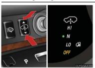
To select a height mode, press  $\triangle$  or  $\nabla$  on the height select switch.
