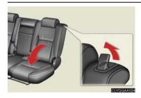
Pull the lever and fold the seatback down until it locks.
