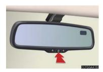
To turn the anti-glare function ON/OFF, press and hold the button for 3 seconds.
