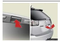
To open the back door, push up the opener and raise the door.
