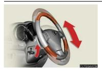
To adjust the steering wheel, pull the lever up while holding the steering wheel, tilt the steering wheel to the desired angle, and release the lever.
