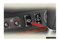
The headlight cleaner can be used only when the ignition switch is in the ON position and the headlights are on.
