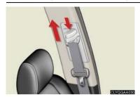
**To raise**: push the anchor upward. **To lower**: depress the button and push the anchor down.
